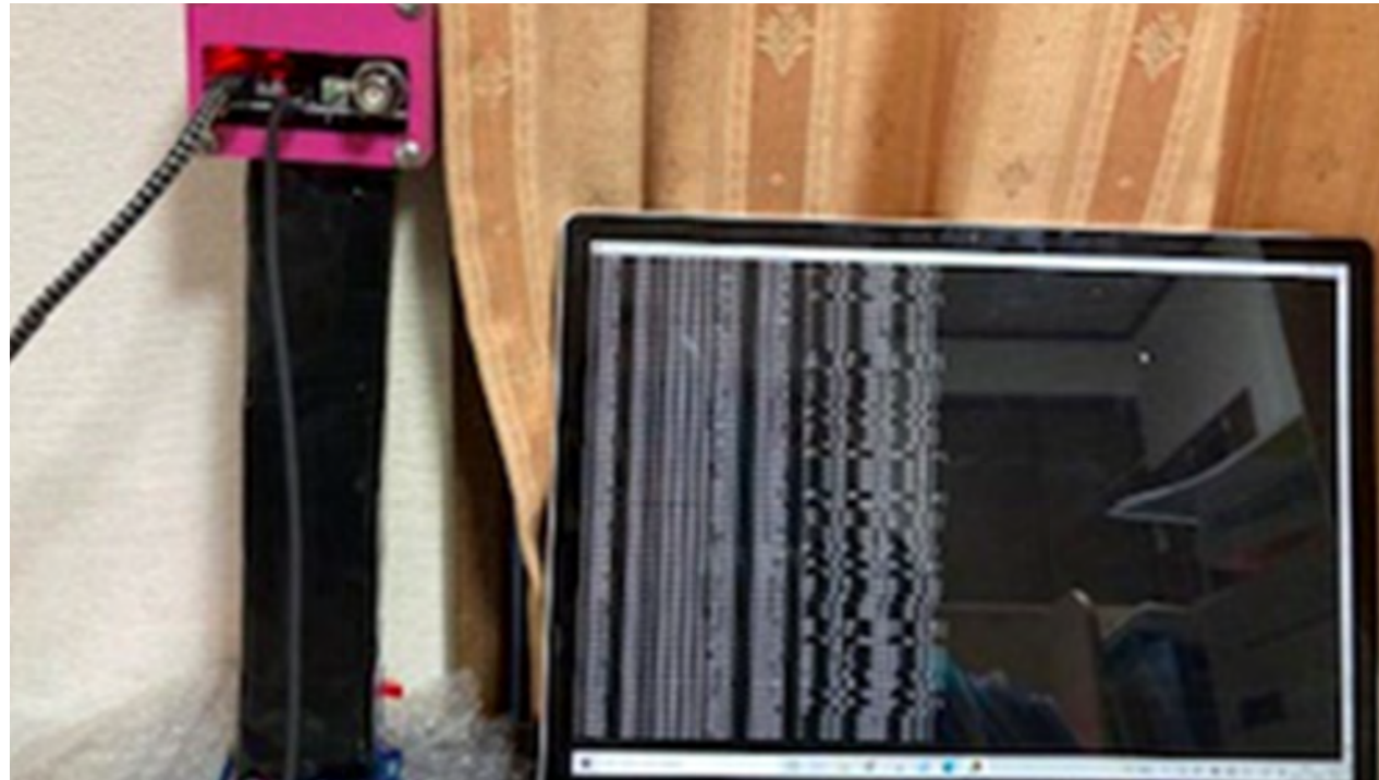
cherenkov detector with acryl block
