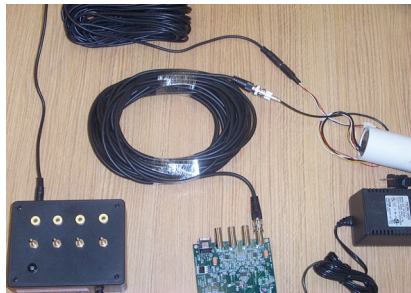
4. PMTs/counters signal cables (4) → DAQ BNC connections: 50 ft. BNC cables
